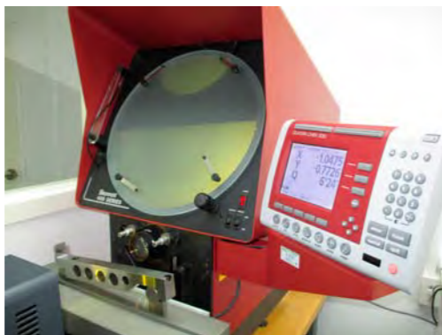
A Starrett Optical Comparator is used for precise non-contact measurement.
