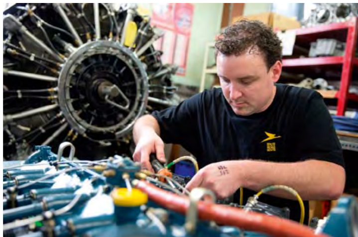
Matt Lee putting the finishing touches to a freshly overhauled Lycoming O-720
