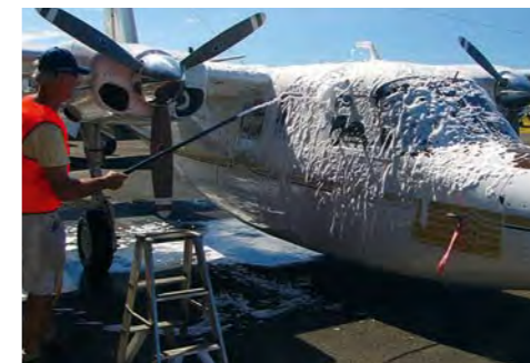
A foam applicator can use less cleaning product, plus save time and improve corrosion protection.
