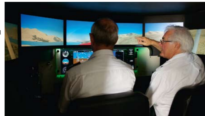
Inside the Redbird. Six wrap-around screens and full motion ensure a most realistic experience.
