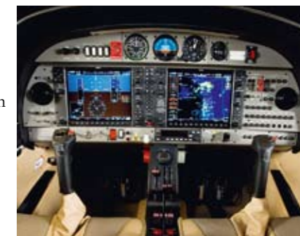
Diamond DA42 cockpit with G1000 avionics
