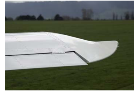
Modified wingtips improve STOL performance. The basic aerofoil is a modified Gottinga 398 profile.
