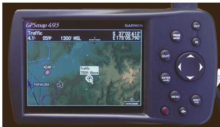
Zaon PCAS can be connected to a compatible GPS, displaying range, direction and relative altitude for nearby traffic whose transponder is being interrogated by radar. You'll be surprised at the number of other aircraft sharing your sky.
