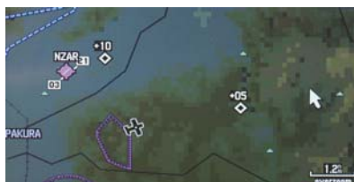
Multiple threats appear as diamonds with relative altitudes displayed, in this case at 500' above and 1000' above.
