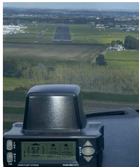
Zaon PCAS operating in stand alone mode on approach to Ardmore. The display indicates nearest traffic on the taxiway 0.3nm ahead and 100' below as well as two aircraft (both recently climbing) in the circuit to our left at relative altitudes of 600' and 900' above.
