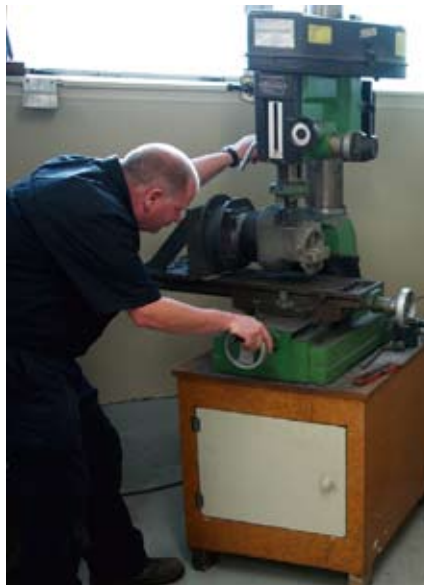
Brett Puddle setting up for port re-facing.
