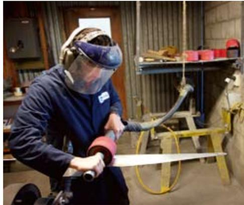
Matt Cox scurfing (surface grinding) a blade surface as part of a propeller overhaul job.
