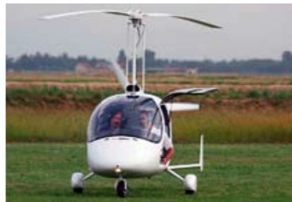
Left: The cabin offers spacious side by side seating for two and full dual controls. Right: Doors hinge at the top and are held by gas struts.
