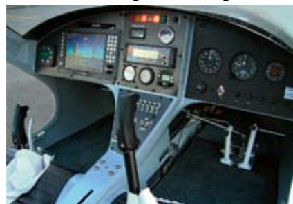
Left: A comprehensive instrument suite includes MGL Avionics EFIS/EMS, Zaon Collision Avoidance and a Mode S Transponder. Right: After the test flight at the Italian factory.
