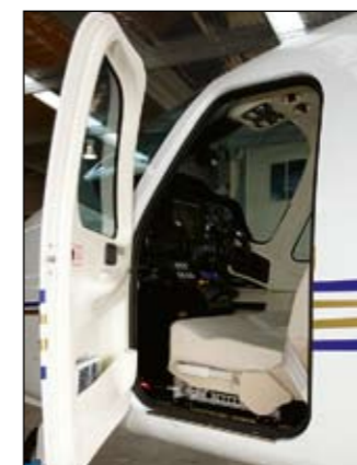
Access to the cockpit is particularly easy. Pilot and Co-Pilot enter by the port side door, the Co-Pilot sliding across to the right hand seat.
