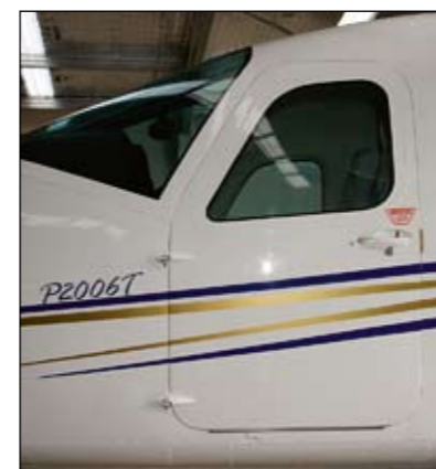
Access to the cockpit is particularly easy. Pilot and Co-Pilot enter by the port side door, the Co-Pilot sliding across to the right hand seat.
