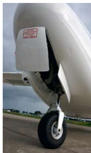
Retractable landing gear is very robust and suitable for less than smooth strips, providing a very comfortable ride during taxiing. Powered by a reversible electric pump, the system is of trailing link design with oleo-pneumatic shock absorbers. The nosewheel is connected by push rods to the rudder pedals.
