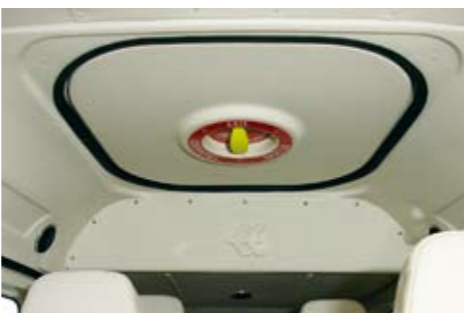
The emergency escape hatch in the roof was a requirement of certification.
