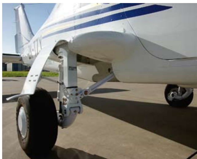
Retractable landing gear is very robust and suitable for less than smooth strips, providing a very comfortable ride during taxiing. Powered by a reversible electric pump, the system is of trailing link design with oleo-pneumatic shock absorbers. The nosewheel is connected by push rods to the rudder pedals.
