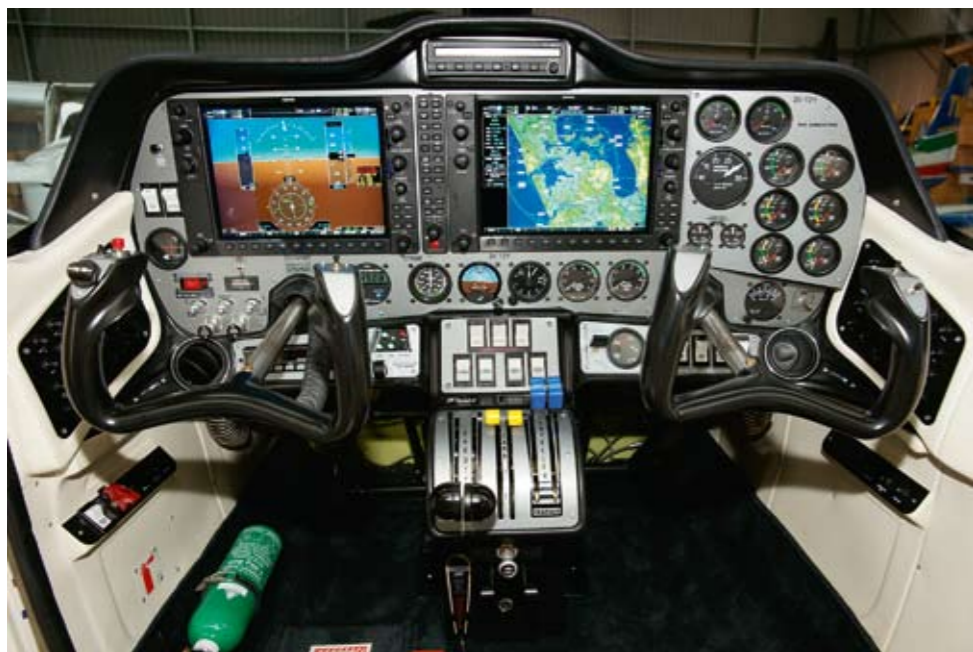
This IFR capable aircraft is equipped with the optional Garmin G950 (essentially a G1000) full glass panel plus auto-pilot. A basic model with traditional instrumentation is also available.
