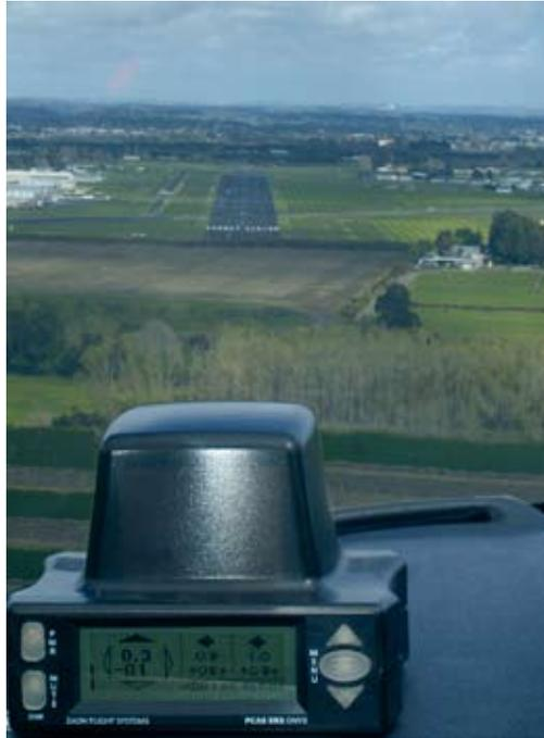
The Zaon XRX, detecting traffic ahead and below (on the runway) and also in the circuit (at left).
