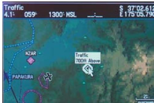
The XRX can interface to a variety of portable GPS units, showing easy to interpret relative traffic positions.
