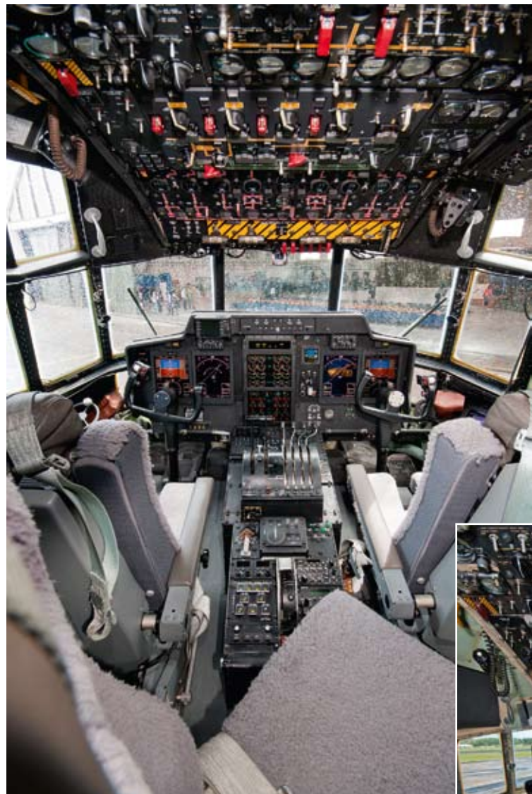
New C-130 LEP NVG compatible glass cockpit.
