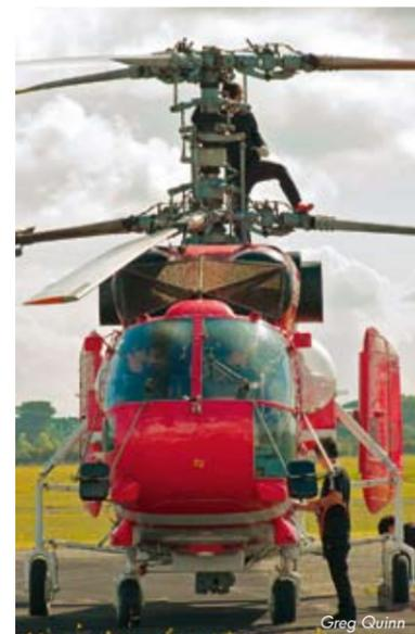
3 Engineers go to work each time the aircraft stops. Note the scale of the rotorhead.
