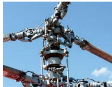
Co-axial rotorhead componentry.
