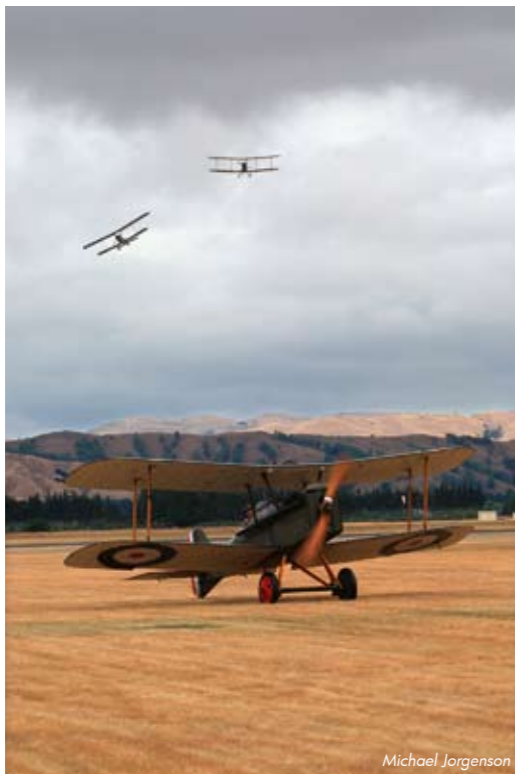
A Royal Aircraft Factory S.E.5a taxiing along the flight line at Hood. Powered by an original Hispano-Suiza Direct drive 180 HP engine, the S.E.5a was the first major project The Vintage Aviator Ltd. undertook.
