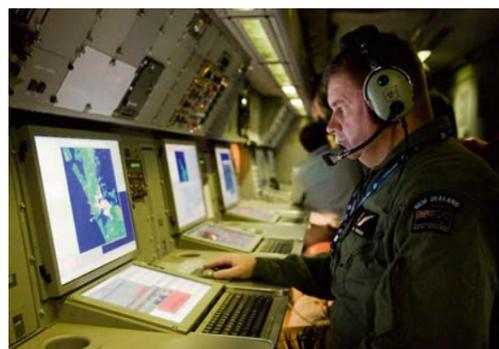
Warrant Officer Rod Simpson operates one of the new tactical crew workstations. Each station is able to operate any of the aircrafts systems to allow maximum flexibility and redundancy. Photo: LAC Grant Amishaw NZDF.
