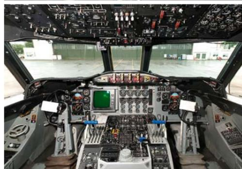
The digital glass cockpit of the new P-3K2 (upper) is a massive improvement on the analogue technology of the legacy aircraft (lower).
