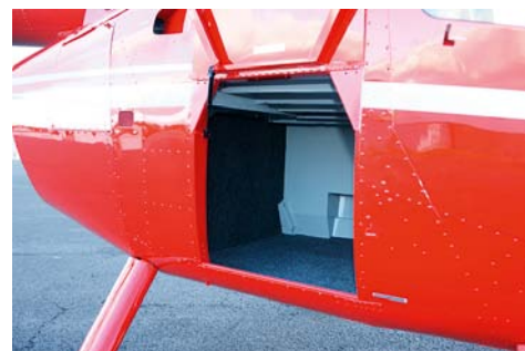
An 18 cubic foot baggage locker will easily accommodate 300lb of suitcases, golf clubs, etc.
