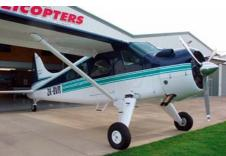
**ZK-BVR** recently flew for the first time in NZ following a complete restoration by Frank Wright and his team from Mount Maunganui. The restoration took just over two years (5000 man hours) to complete and includes a Sealand cabin extension, new forward cabin struts, lifetime wing struts, tip tanks, and much more. An all new interior has been fitted with 8 place leather seating, interior lighting, wool carpets,
