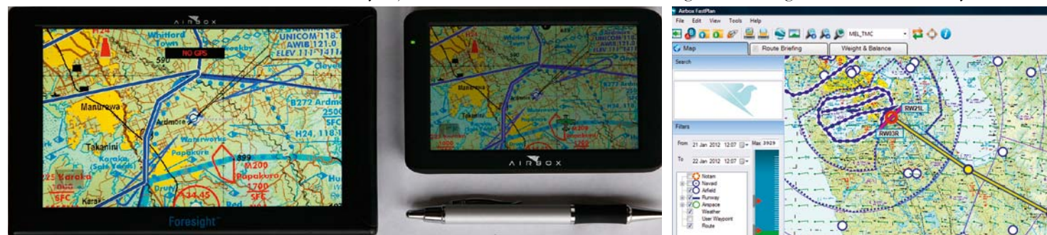
Left and centre: Foresight Superbright and Clarity 2 side by side. The photo was taken outdoors on a bright day in slightly shaded conditions. At right is part of a screen capture of the Airbox Fastplan software for PC based flight planning (downloadable to the device) that is free with the Clarity and Foresight.
