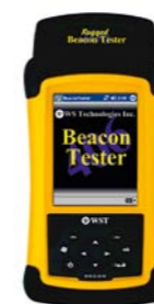
Emergency Beacon Testing Equipment
