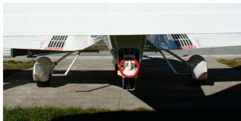
A tow hook is certified for gliders up to 700 kg and banners up to 140 m 2 .
