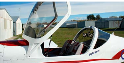
The Harmony canopy opens forward for easy access to a spacious cockpit.
