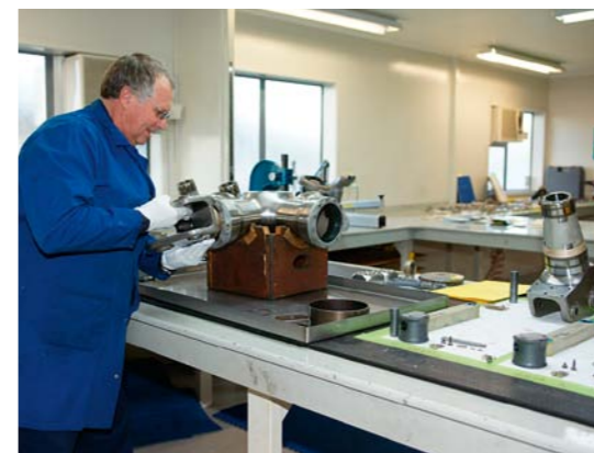
Loffie Schoeman working on a BK117 rotor head.
