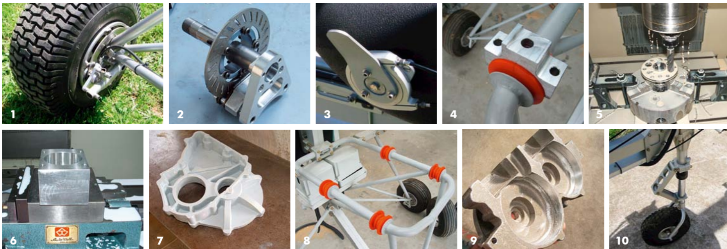
1. Dominator suspension with disc brake package fitted. 2. Disc brake components. 3. Multi cable push-pull throttle quadrant. 4. Engine mounting system component. 5. CNC machining a gearbox output flange. 6. RFD rotor-head bearing block. 7. 3D modelled, machined pattern for casting. 8. Subaru EA81 engine frame on Dominator gyro. 9. Two stroke crankcase casting in CC601-T6 ready for machining. 10. Front oleo with damped castering wheel.
