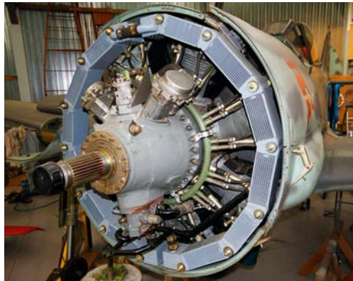
The 14 cylinder Russian Shvetsov ASH-82 engine provides the Flug Werk FW 190 with 1850hp.
