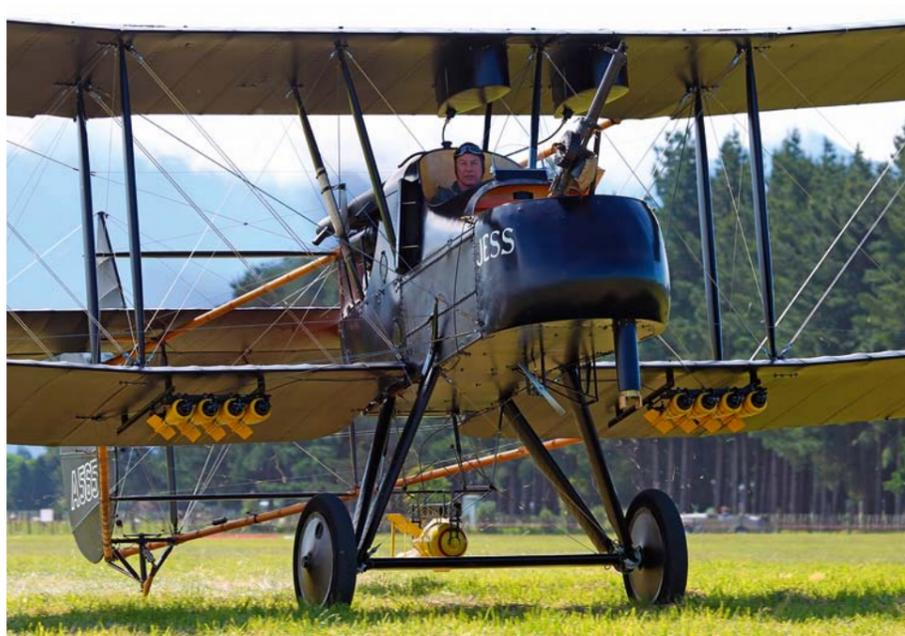
Gene De Marco heads out in the FE.2b night bomber. The tubular shaped thing under the front cockpit section is the aiming system for the 9 bombs that make up the bomb load. It is great to see one looking so authentic.
