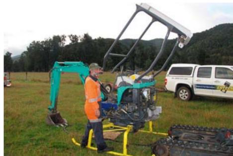
The canopy rotates onto the track unit.
