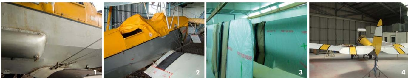
1&2: Pre restoration. 'Crazy cracks' were present in the paint everywhere. 3: Wings masked for the black stripes. 4: Nearing completion during re-assembly.
