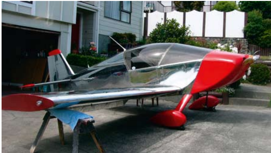
Sonex ZK-RMK is an example of an amateur-built Light Sport Aircraft.
