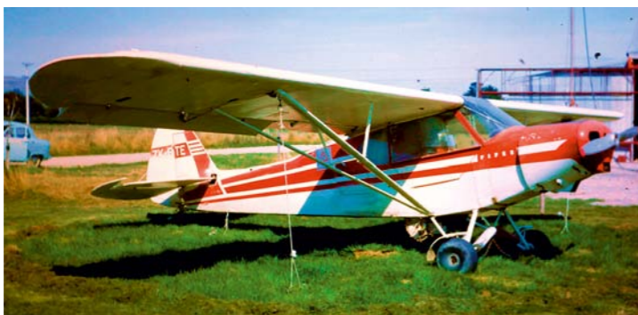
ZK-BTE was operated by Aerial Farming, Aerial Work and Airspread and is identical to Central Aviation's (Roxburgh) two Super Cubs BNX/BKM, flown by Doug Johnson (Roxburgh) and Peter Bevan (Clyde) that I used to watch in awe at work in the mid to late 1950s. Note the chain strung between the wheel legs of BTE which is there to prevent the legs from spreading (and collapsing) under weight on rough ground. (Dave Paull Photo - 1963)
