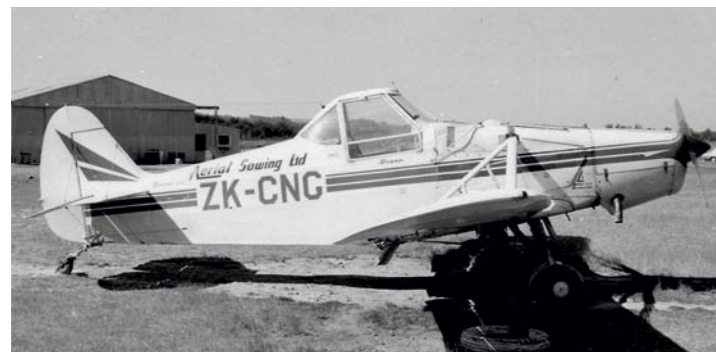
Pawnee PA-25-235B ZK-CNG (C/n 25-3624), which flew with Aerial Sowing and Airwork, was one of 49 purpose-built Pawnee topdressers to arrive here from 1962. This photograph was taken at Timaru by Bob Kerr in its heyday. CNG is today with the Canterbury Gliding Club as a towplane with a 250hp Lycoming engine under the bonnet. Airwork (NZ Importers) was one of our biggest users of the Pawnee, having 14 of them on line at one time. (John Nicolson Collection)
