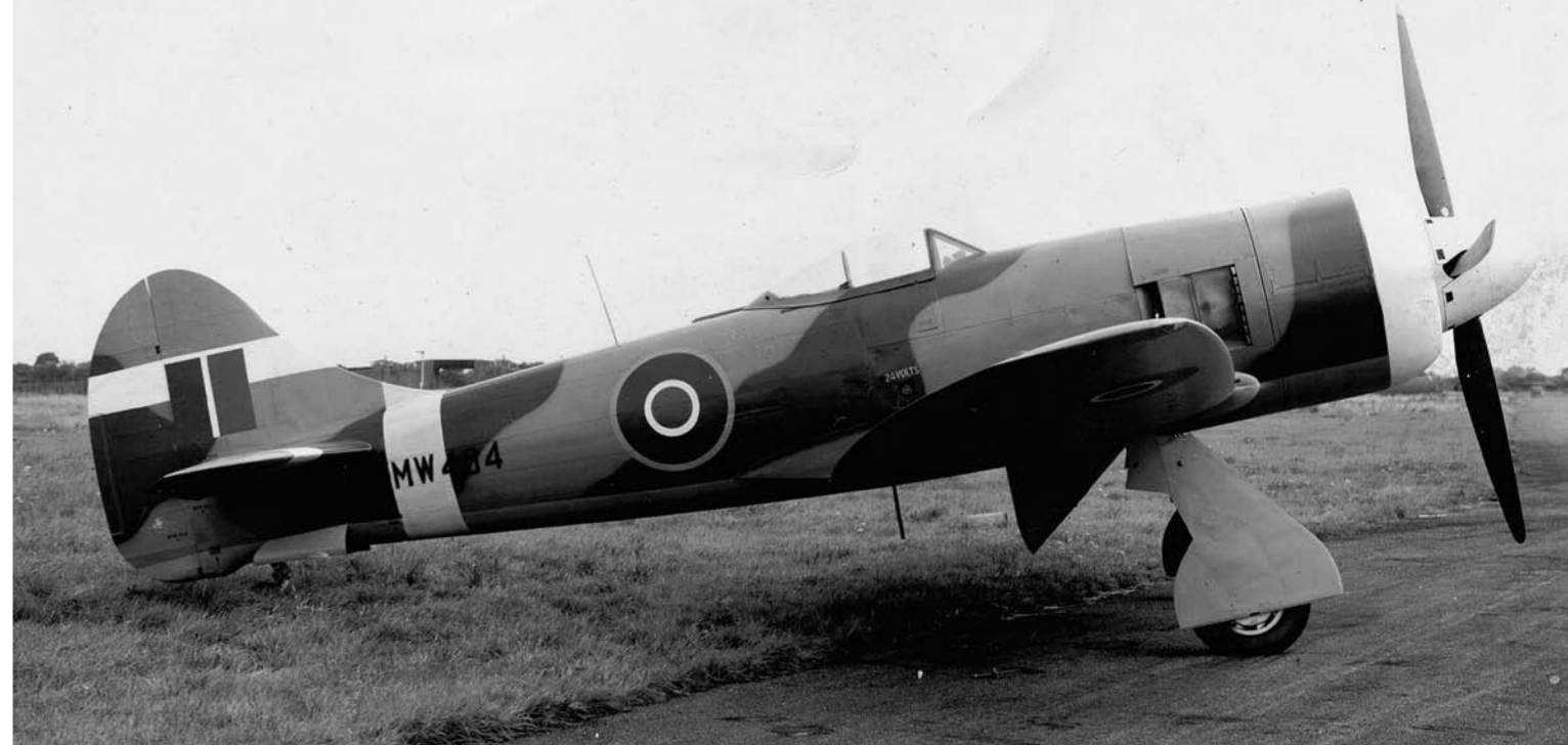
A WWII image of the exact same type, this example designated MW404, being a Hawker Tempest Mk.II with Bristol Centaurus V engine.
