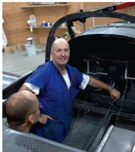
Neil (centre) and Lapo in the Furio fuselage setting up the alignment of rudder cable fittings.
