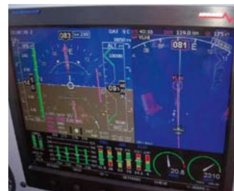
Furio in cruise mode: 2310rpm, 20.8", 175ktsGS, 166ktsTAS at 9530' using just over 30lph.
