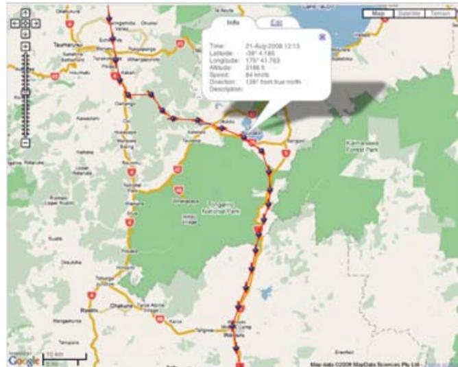
spidertracks screen image showing internet based aircraft tracking in action
