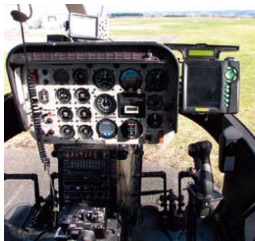
The 407 office. Extras include additional radios and a TracMap GPS system.
