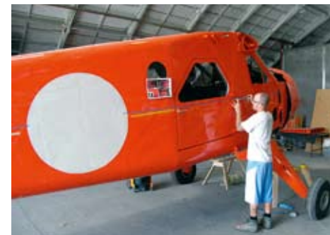
The process of detailing began with preparation for stripe painting on the fuselage.
