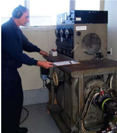
'Chuck' Osborne at work in the Aeromotive Electrical Bay: Running up a freshly overhauled generator (above) and making repairs to the circuitry of a rudder trim actuator (below).
