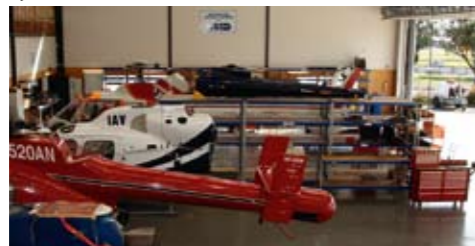
Racks in each bay offer dedicated space for aircraft cowls and parts, keeping them off the floor.
