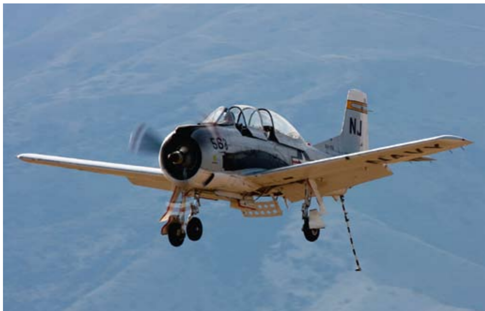
Converted for aircraft carrier operations with a tail hook and stronger undercarriage, the Navy T-28C model was first flown in 1955. Gavin Conroy photograph from Warbirds over Wanaka 2008.
