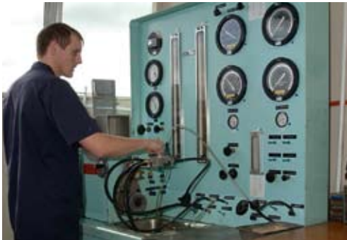
Thomas Kiddle testing the diaphragm section of a RSA7AA1 from a Hughes 300 engine.
