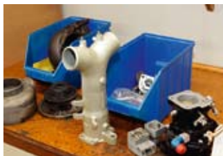
Work in progress l to r: Garrett Air Research turbocharger under repair; TCM fuel injection system under overhaul; Marvel Schebler carburettor also in for overhaul.
