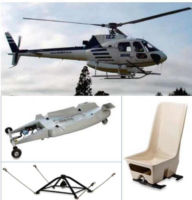
AS350 role equipment includes a Carbon Fibre Spray System, Seat Slider and Cargo Hook Swing Frame. The latter two are also suitable for the AS355.
