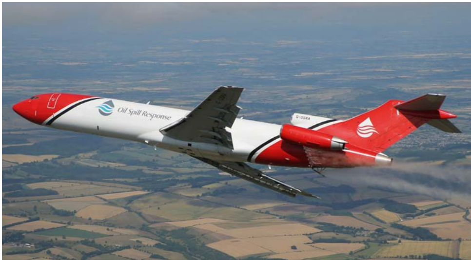
Note the large boom on the back for spraying oil dispersant as demonstrated here but with water.
