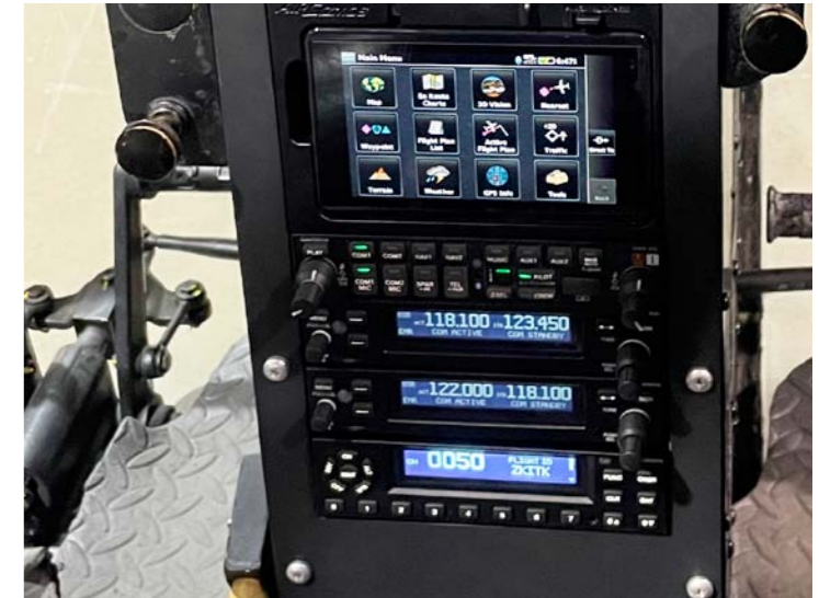
A recent avionics upgrade completed by Oceania Aviation on a B206 Long Ranger.
