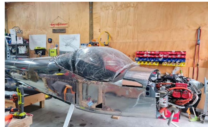
Riveting around the canopy after trimming to fit. Engine install mostly complete.
