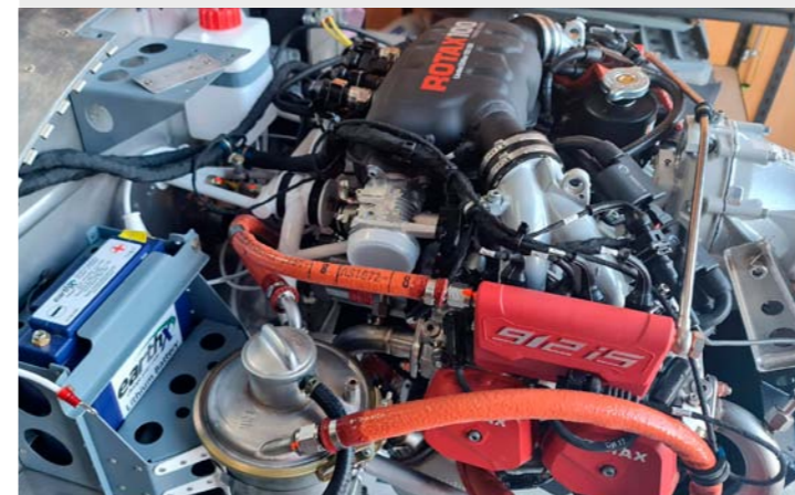
A tidy Rotax 912 iS engine installation.
