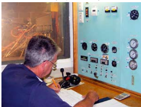
A Lycoming O-320 has just completed a carburettor change. John Williams writes up the Test Cell report card.
