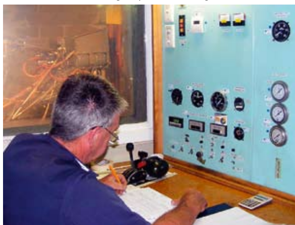
A Lycoming O-320 has just completed a carburettor change. John Williams writes up the Test Cell report card.
