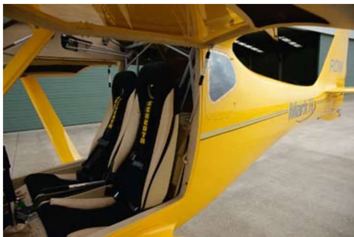
Doors lift upwards for easy access. The tubular steel cockpit frame can be seen. Note also the access door to the luggage area and the towhook under the tail.
