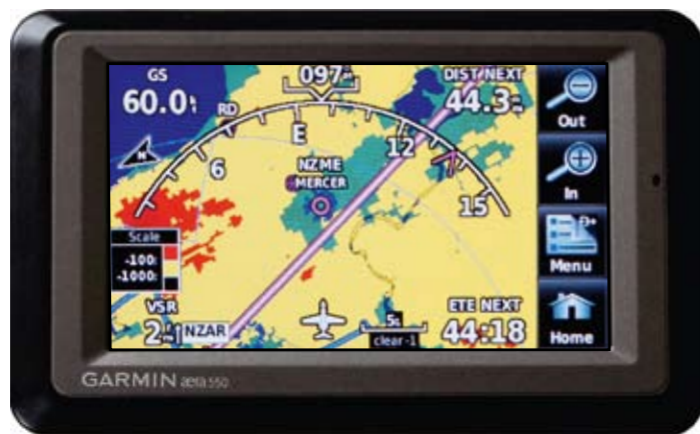
Typical track and route display, in this case with terrain background shading. Points of interest can be selected by touching them on the screen.
