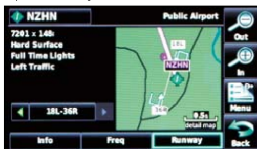
The Hamilton arrival page. Note the appearance of Info, Frequency and Runway buttons on screen.
