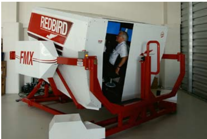
The Redbird FMX Full Motion Simulator at Ardmore. The motion platform is all electric and quite capable of inducing spatial disorientation when asked to.
