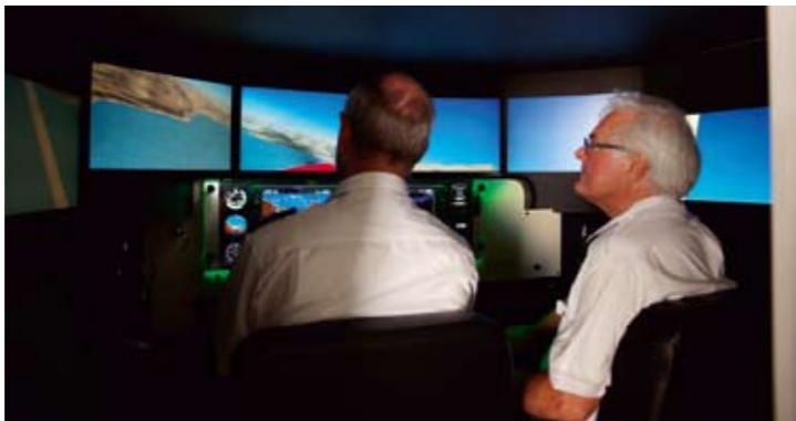
Inside are six wrap-around monitors. Realistic flight controls and instruments can be easily exchanged for different aircraft and avionics configurations.
