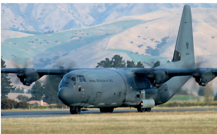
The lack of underwing fuel tanks is a give away for a J model.
