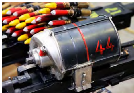
The replica ammo feeder for the 20mm cannons.
