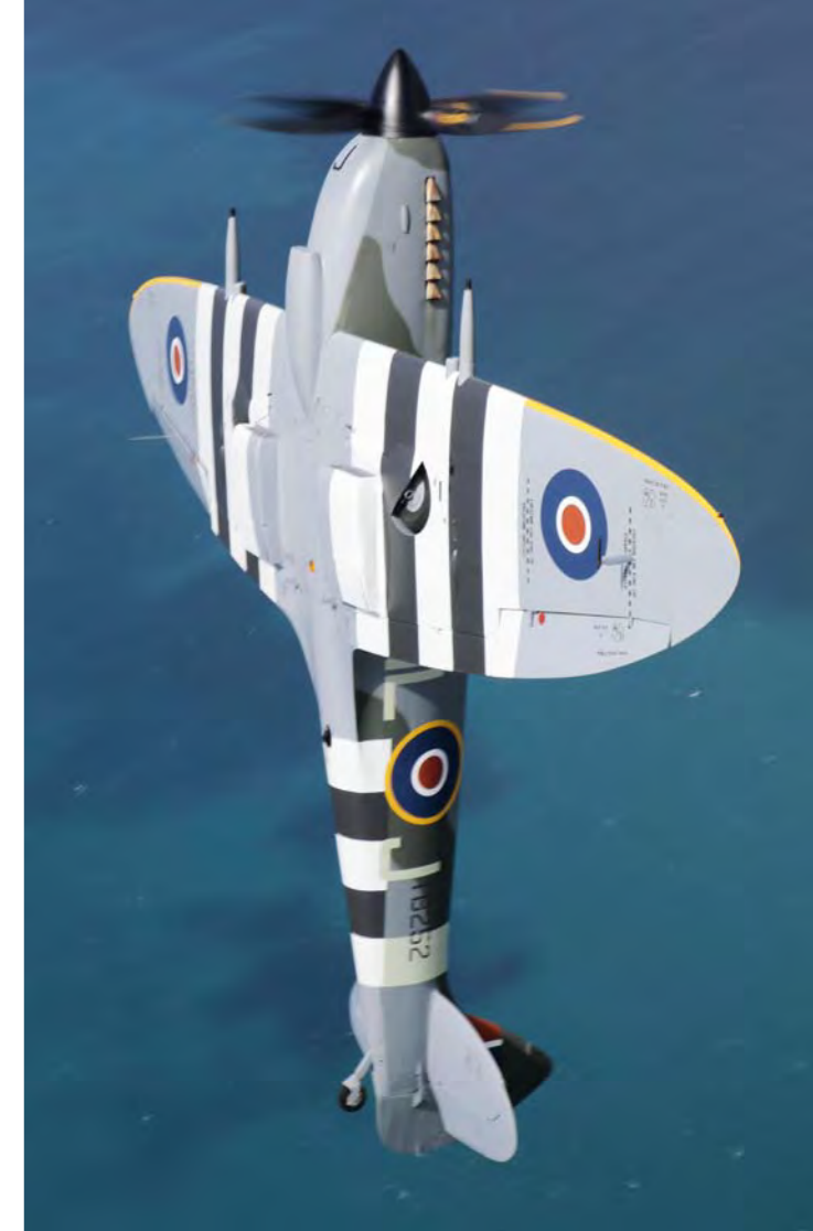
The blown canopy supports rear visibility, important to avoid becoming a target.
