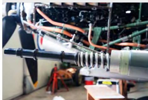
Replica cannons include massive recoil springs.
