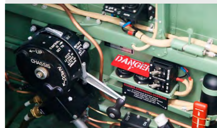
Under the danger cover are buttons to destroy the Friend or Foe Identifier in case of falling into enemy hands. (Small charges were installed in the casing.)
