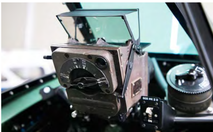
Graduations on the gunsight dial cover a wide range of enemy aircraft.
